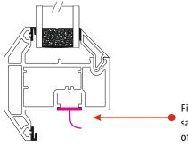
Fit a Sash Spring to the sash on the center line of the stay fixing area
